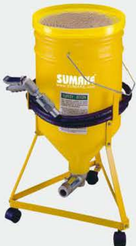
SB-215 Sand Blaster Bucket Capacity: 5 Gallons Bucket Material: LLDPE Bucket Thickness: 5mm Bucket Diameter: \phi 280mm Overall Height: 700mm Packing Dimensions: 570(L) x 330(W) x 330(H)mm Nozzle Size: 5/16" Option: 3/16" .3/8" .1/2"
